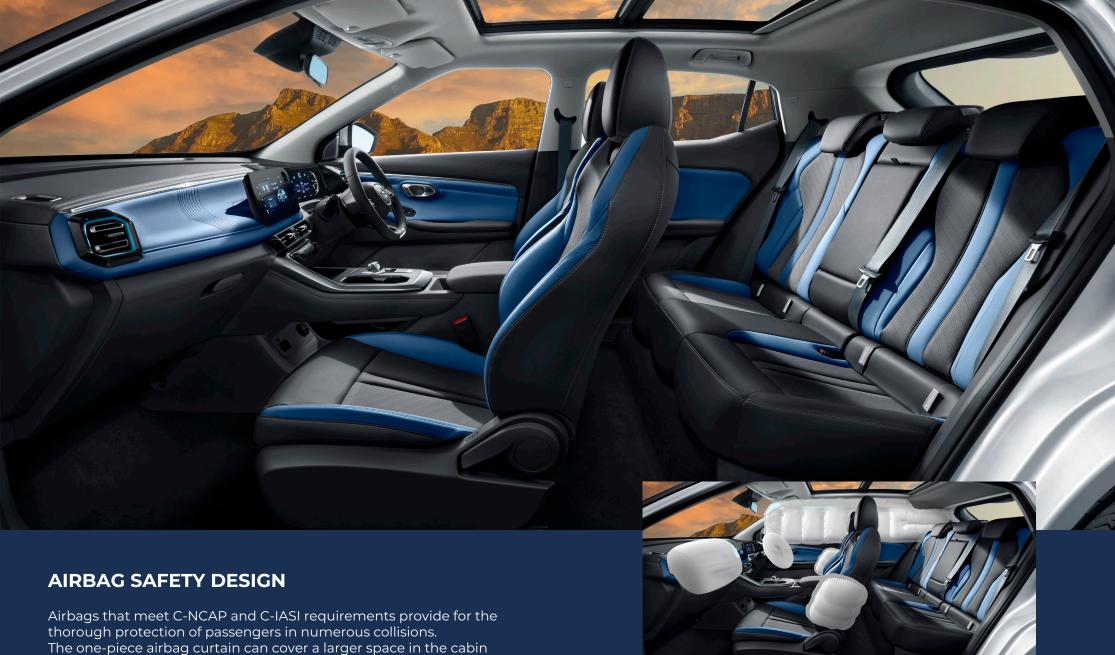
The one-piece airbag curtain can cover a larger space in the cabin and comes with an extra-long 6-second pressure retention feature, providing more comprehensive protection.
